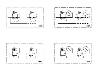
FR19 = Manifold regulator with relieving and without manometer FR20 = Manifold regulator with relieving and manometer FR21 = Manifold regulator without relieving nor manometer FR22 = Manifold regulator without relieving and with manometer
